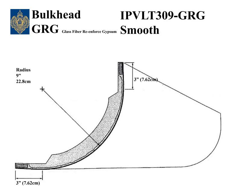
\* assembly required, all measurements are approximate only Secure with Screws, Tape & Mud Seams
