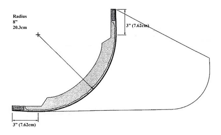
\* assembly required, all measurements are approximate only Secure with Screws, Tape & Mud Seams
