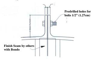
Each Section has an exterior bolt flange, pre-assembled and fitted before shipping
