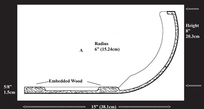
**MATERIAL: NeoPlaster-GRGTM** Alpha Gypsum, cement, water, reenforced with glass fibers. Lite weight 2-3lbs per square foot. Meets ASTM-E84 Fire rated. Odorless and emission free. Interior use only in dry areas. Made in molds, tape & mud seams.
