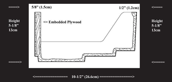
MATERIAL: NeoPlaster-GRGTM Alpha Gypsum, cement, water, reenforced with glass fibers. Lite weight 2-3lbs per square foot. Meets ASTM-E84 Fire rated. Odorless and emission free. Interior use only in dry areas. Made in molds, tape & mud seams.
