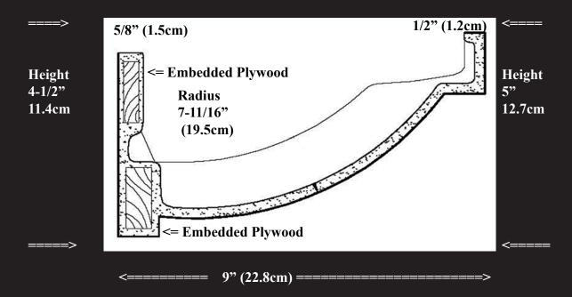
MATERIAL: NeoPlaster-GRGTM Alpha Gypsum, cement, water, reenforced with glass fibers. Lite weight 2-3lbs per square foot. Meets ASTM-E84 Fire rated. Odorless and emission free. Interior use only in dry areas. Made in molds, tape & mud seams.
