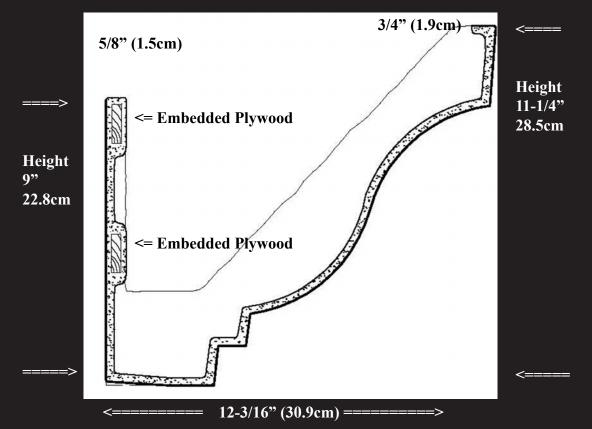
MATERIAL: NeoPlaster-GRGTM Alpha Gypsum, cement, water, reenforced with glass fibers. Lite weight 2-3lbs per square foot. Meets ASTM-E84 Fire rated. Odorless and emission free. Interior use only in dry areas. Made in molds, tape & mud seams.
